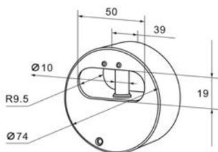
Lock body - cast iron, with protection of the shackle from breaking
