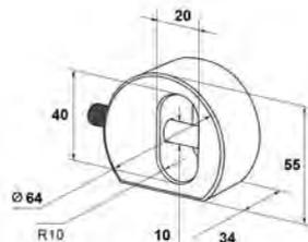
Lock body - cast iron, with protection of the shackle from breaking
